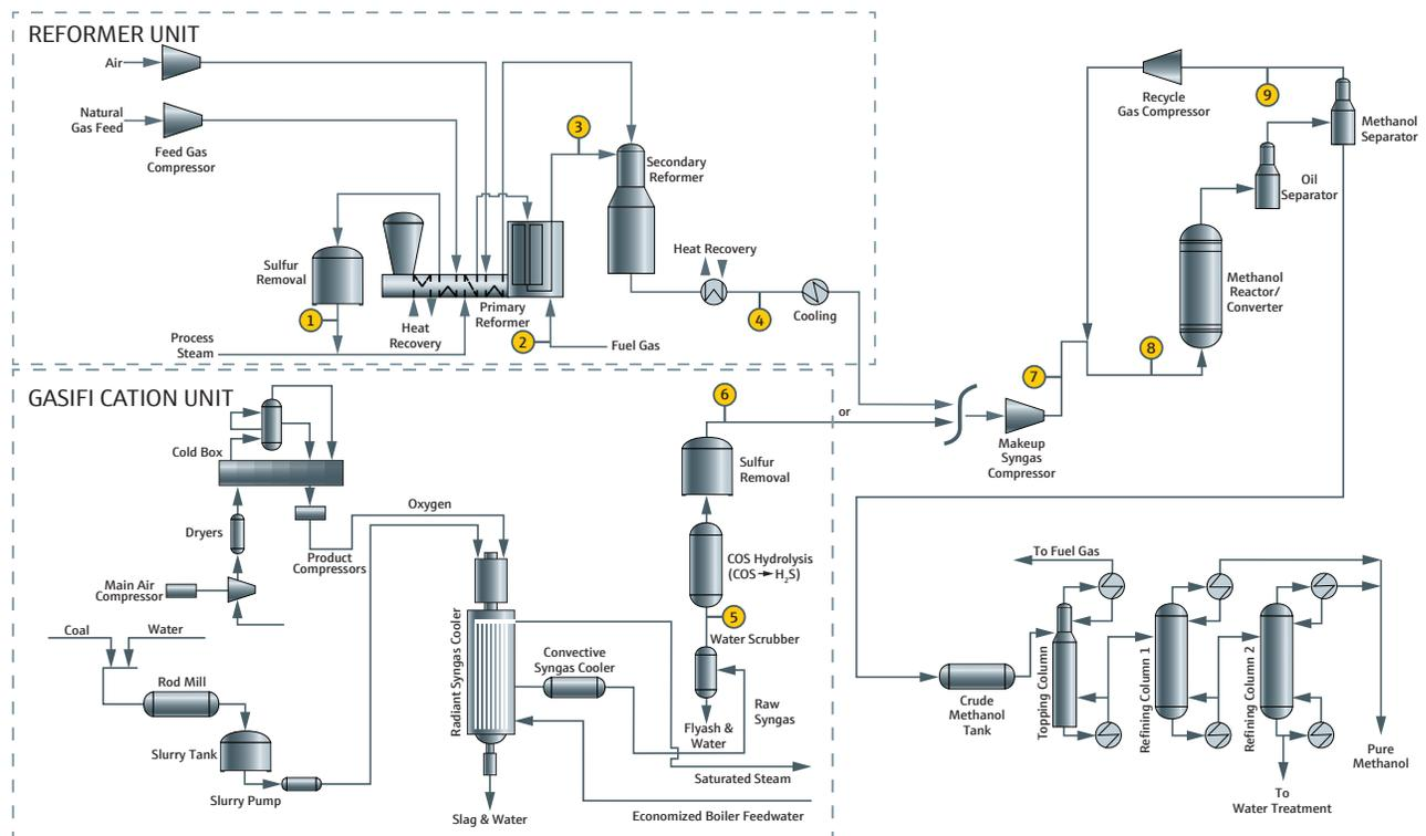
Figure 1: A Simplified Process Diagram Showing the Main Process Units in a Modern Methanol Production Plant
